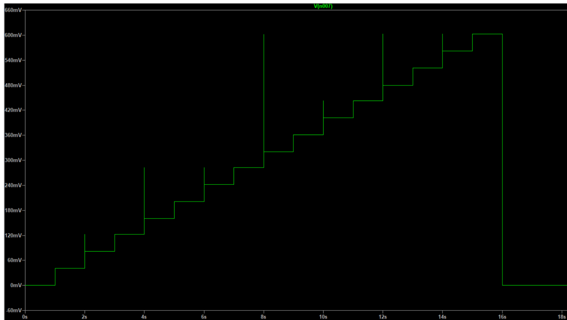
Figure 2: LTspice simulation of 4-bit DAC
