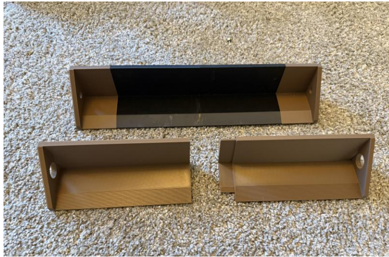
Figure 8. 3D-Printed End-Effector Sections Laid Out Before Assembly
