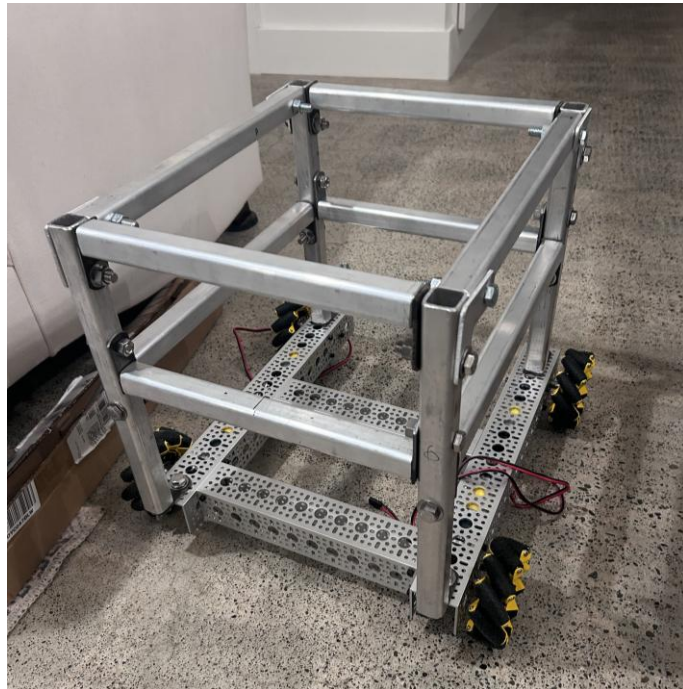
Figure 26. Multi-Level Frame Assembled with Mecanum Wheels
