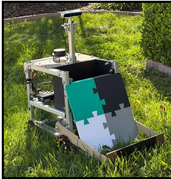
Figure 1: Completed LitterBot Prototype with Integrated Drive, Collection, Sensing, and Control Subsystems
