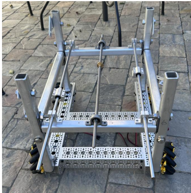
Figure 25. Chassis Assembly Outdoors - Lead Screw and Linear Slides Visible
